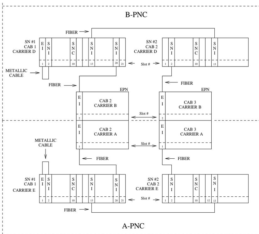
**Figure 9-30. Center Stage Switch Configuration with Duplicated PNC**
