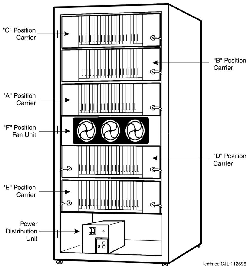
Figure 9-14. Typical Multi-Carrier Cabinet with 649A Power Units
