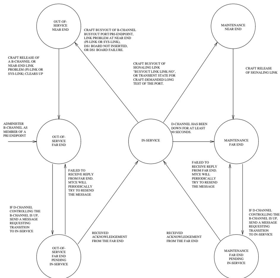
Figure 9-60. Common Progressions in PRI Endpoint Service States
