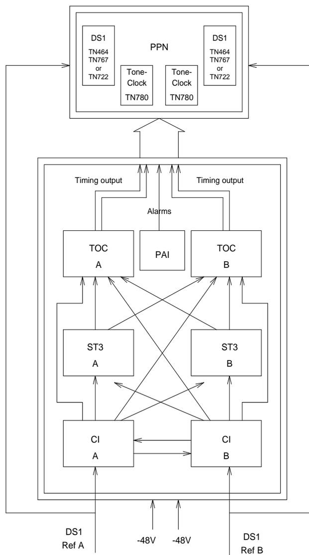
Figure 9-75. Stratum 3 Clock Hardware Configuration
