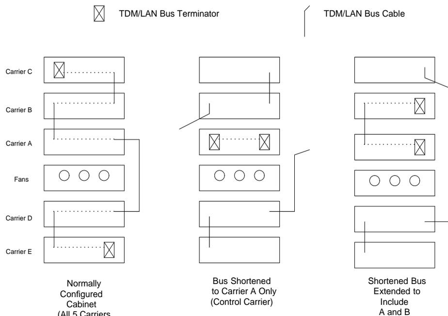
**Figure 9-93. Carrier Rewiring Example—Rear View of Five-Carrier Cabinet**
