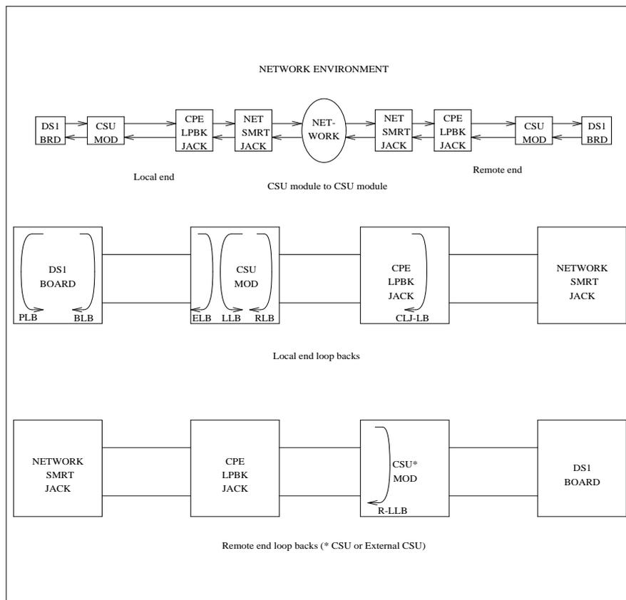
**Figure 9-94. High Level Overview Of Loopback Points**
