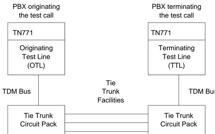
**Figure 9-50. ATMS Tie Trunk Test Call**
