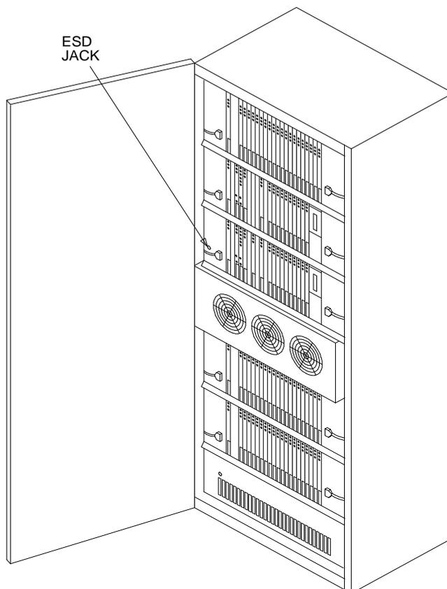
Figure 5-1. Multi-Carrier Cabinet ESD Grounding Wrist Strap Jack
