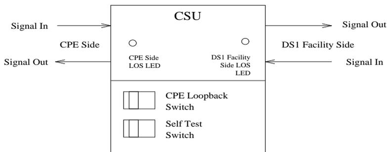
Figure 9-19. Typical CSU Maintenance Capabilities
