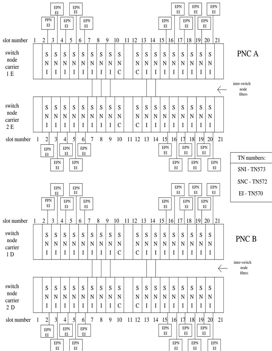
**Figure 9-70. CSS Configuration with Duplicated PNC and 4 Switch Node Carriers**
