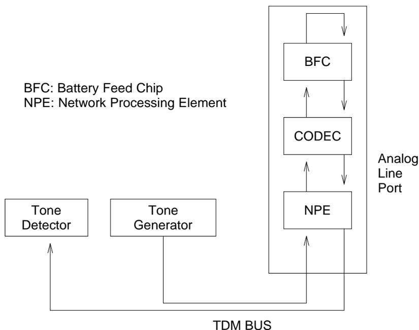
**Figure 9-1. Analog Loop Around and Conference Test**
