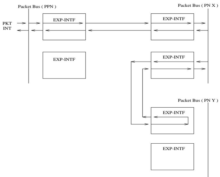
**Figure 9-40. Expansion Interface Packet Interface Test-EPN to EPN link**
