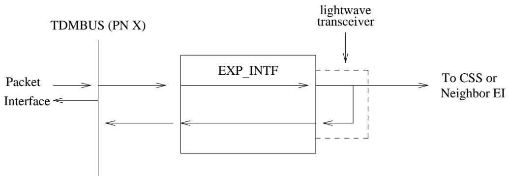
Figure 9-35. Packet BUS Lightwave Transceiver Looparound—PPN only
