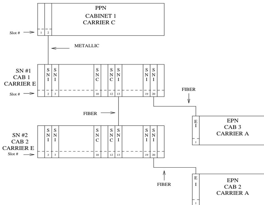
**Figure 9-29. Center Stage Switch Configuration with Simplex PNC**
