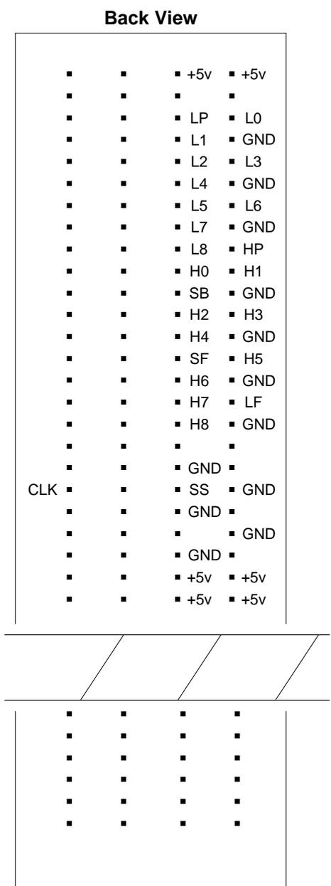
**Figure 5-13. Packet Bus Leads on the Backplane**
