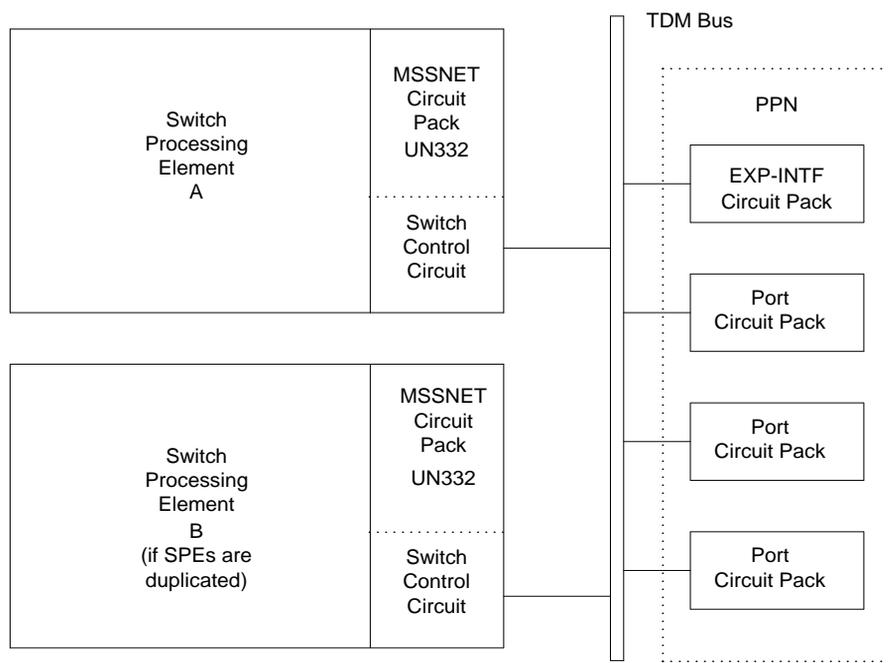
Figure 9-76. Switch Control Connectivity
