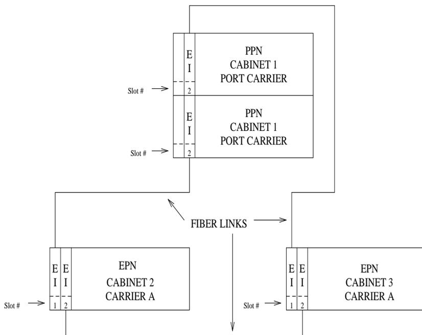
Figure 9-27. Direct Connect Configuration with Simplex PNC
