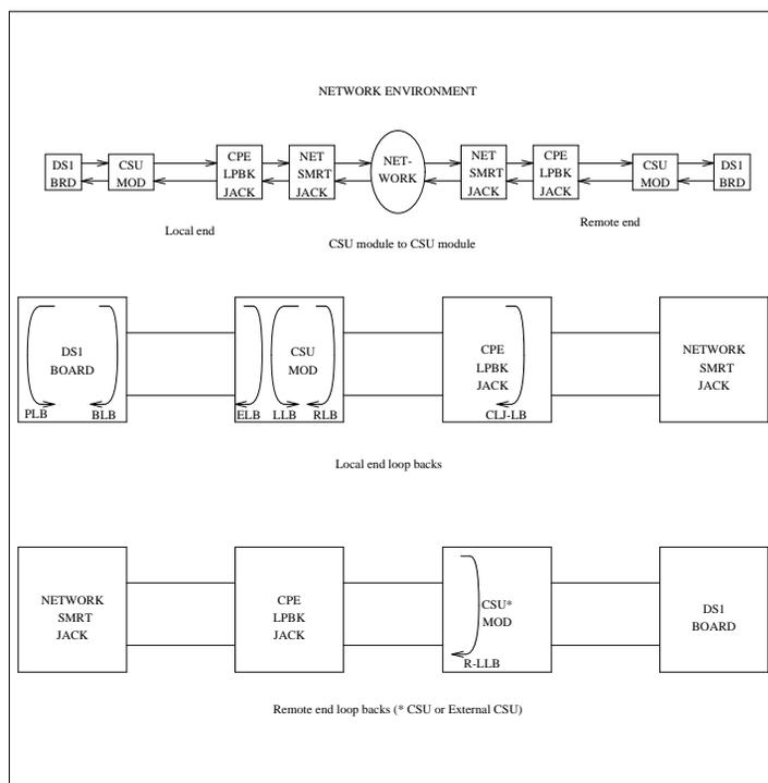
Figure 9-16. High Level Overview Of Loopback Points
