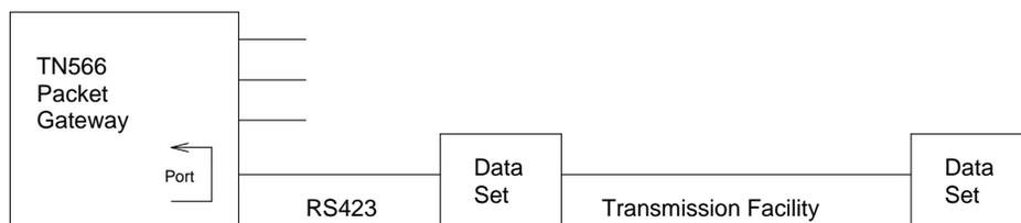
**Figure 9-61. Packet Gateway Port Local Loop-Around Test**
