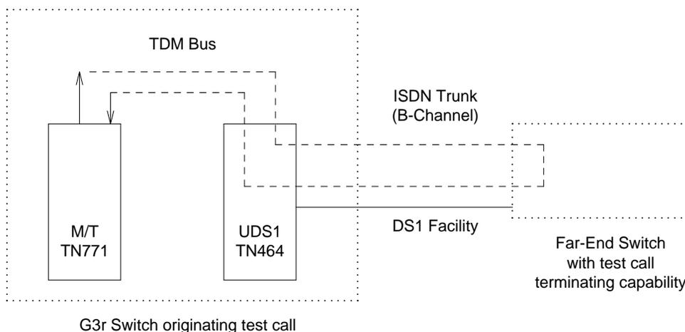
**Figure 9-43. Outgoing ISDN-PRI Test Call**
