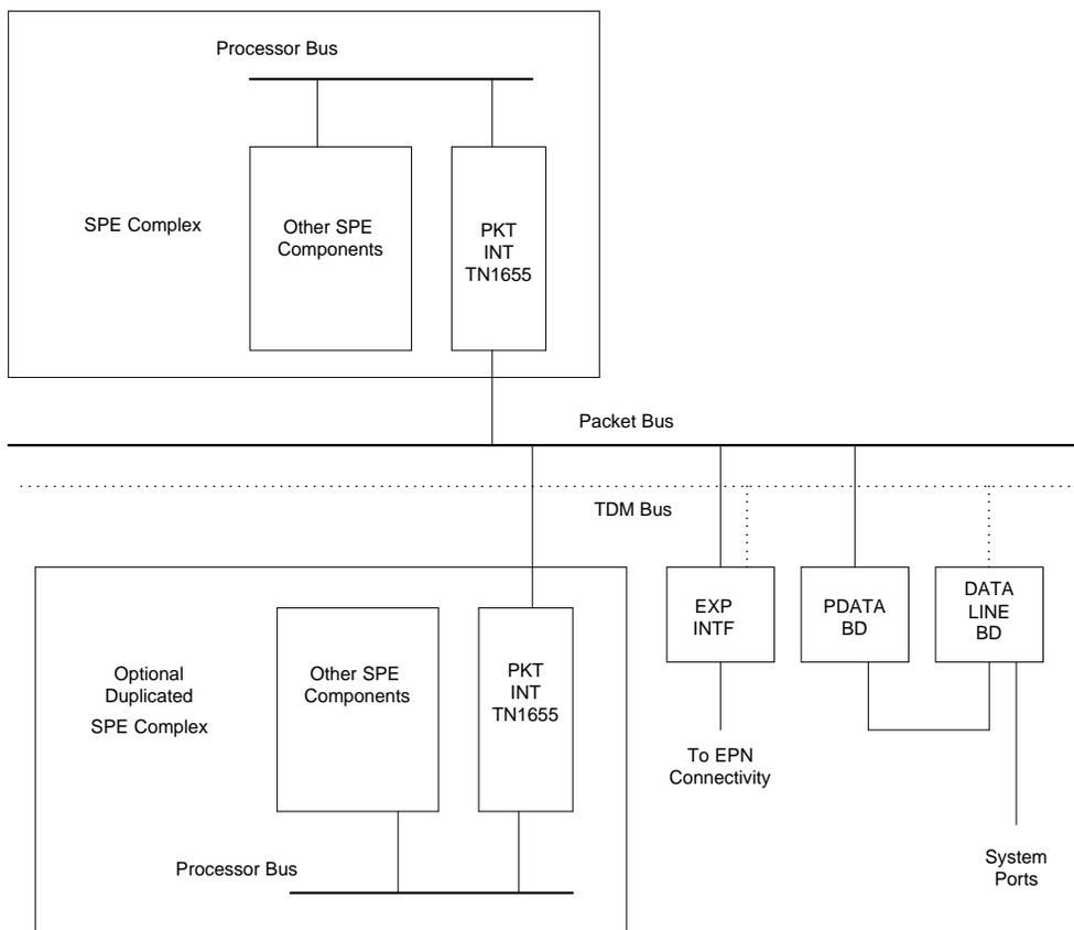
**Figure 9-64. Packet Interface Connectivity**
