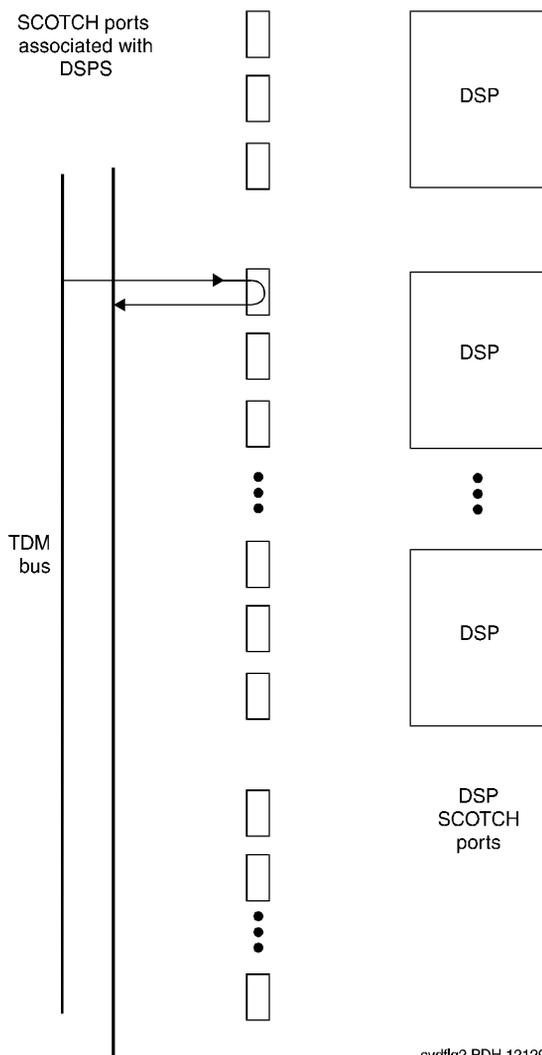
Figure 9-98. VC Circuit Pack DSP Port Local TDM Loopback Test
