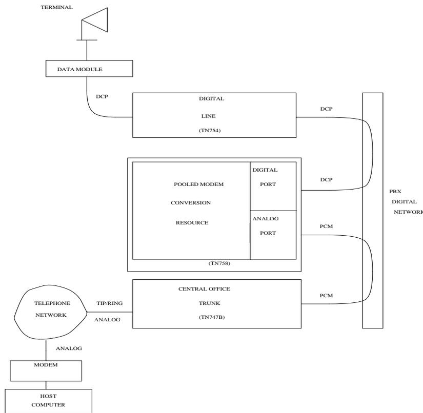
Figure 9-47. Typical Modem Pool Switched Connection with Integrated Pooled Modem
