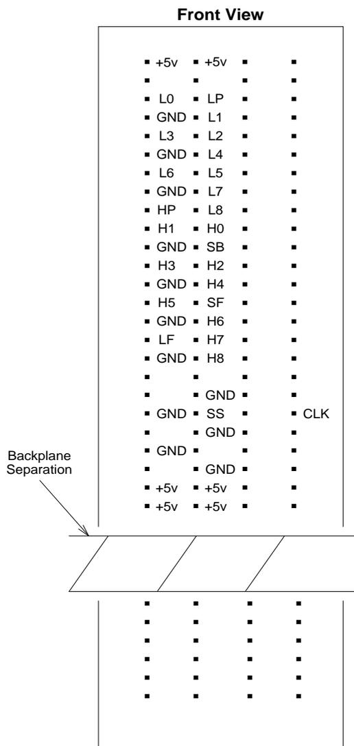
**Figure 5-12. Packet Bus Leads on the Backplane**
