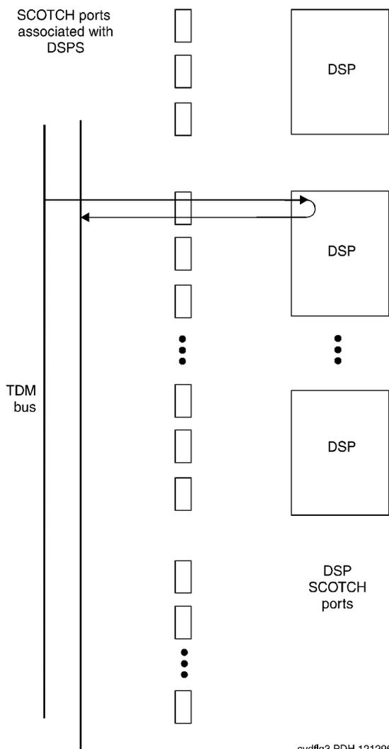
Figure 9-99. VC Circuit pack DSP Port DSP Looparound Test
