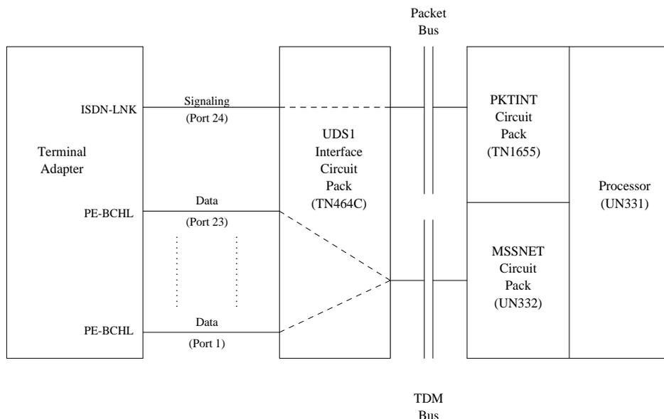
**Figure 9-59. PRI Endpoint Port Interactions**
