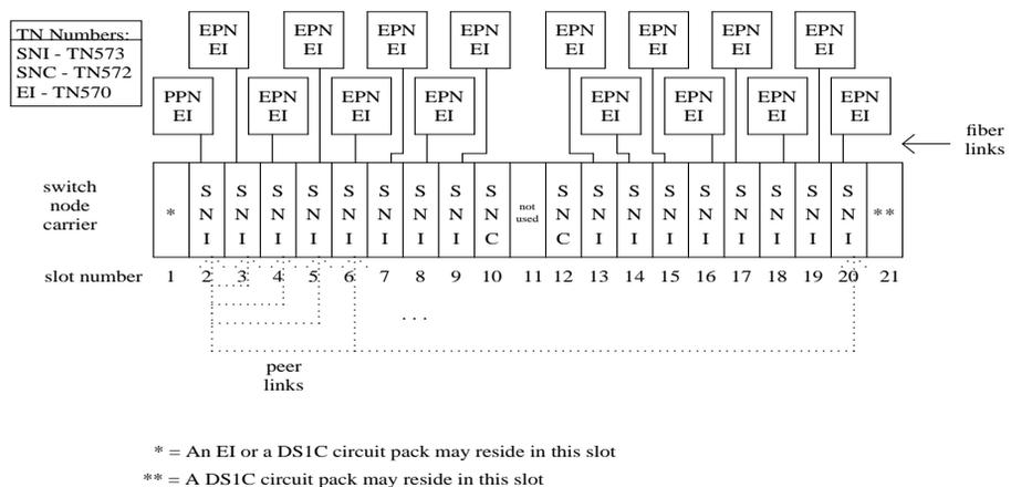
**Figure 9-69. CSS Configuration with Simplex PNC and 1 Switch Node Carrier**
