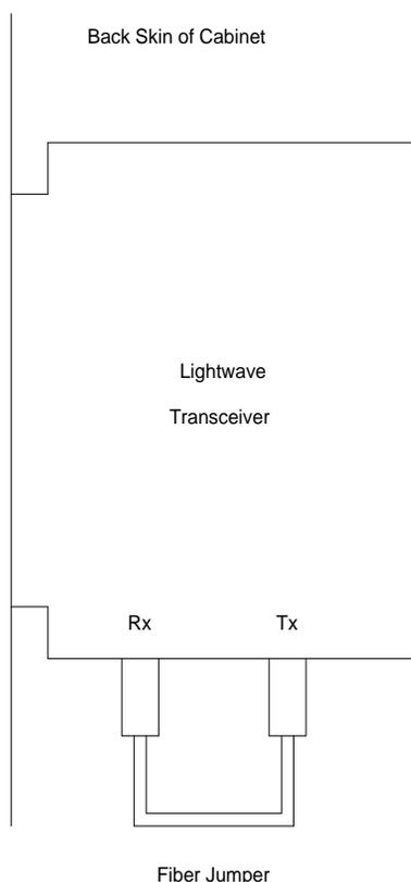
**Figure 9-72. Interconnection of Lightwave Transceiver Transmit/Receive Jacks**
