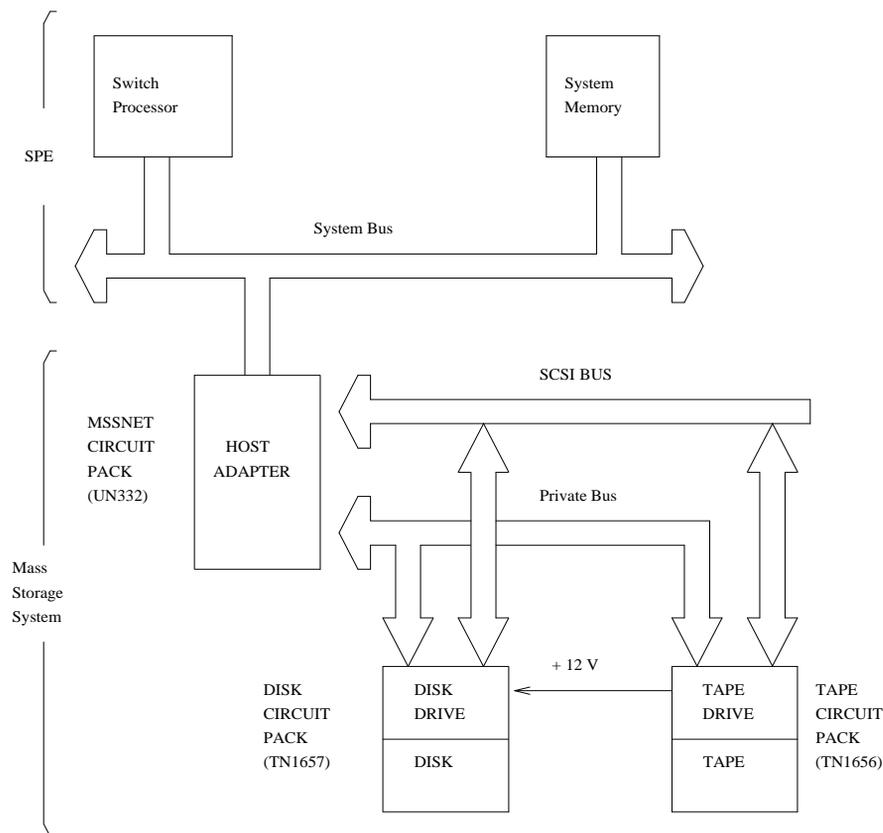
**Figure 9-15. Mass Storage System Interactions**
