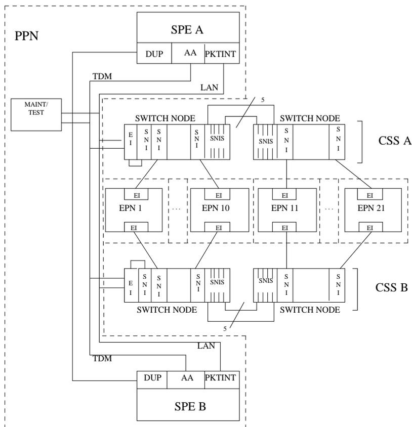
Figure 9-66. Duplicated PNC with Center Stage Switch
