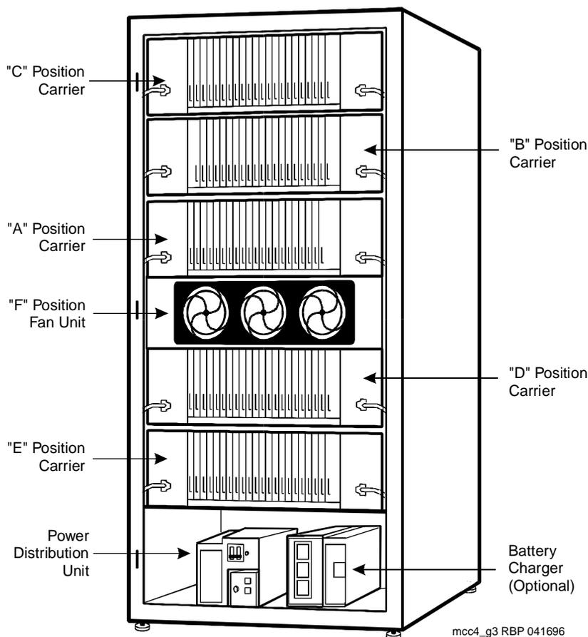
Figure 9-9. AC Power Distribution in Multi-Carrier Cabinets
