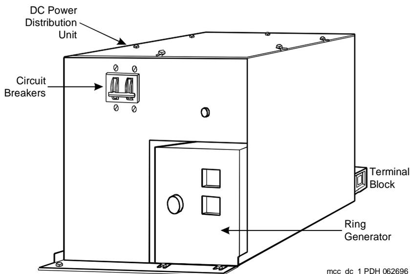
**Figure 9-13. DC Power Distribution Unit (J58890CF-2) — Front**
