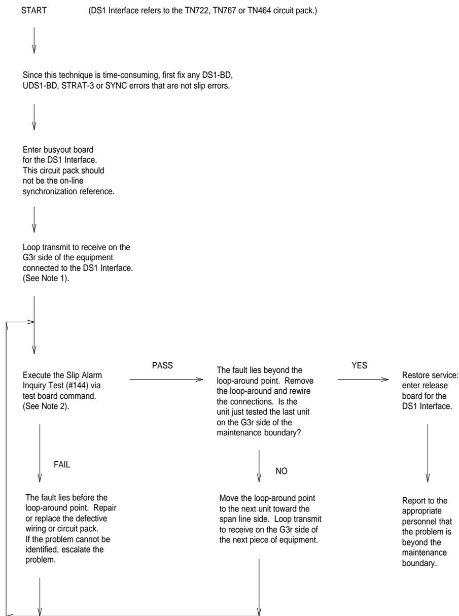
Figure 9-87. Facility Fault Sectionalization
