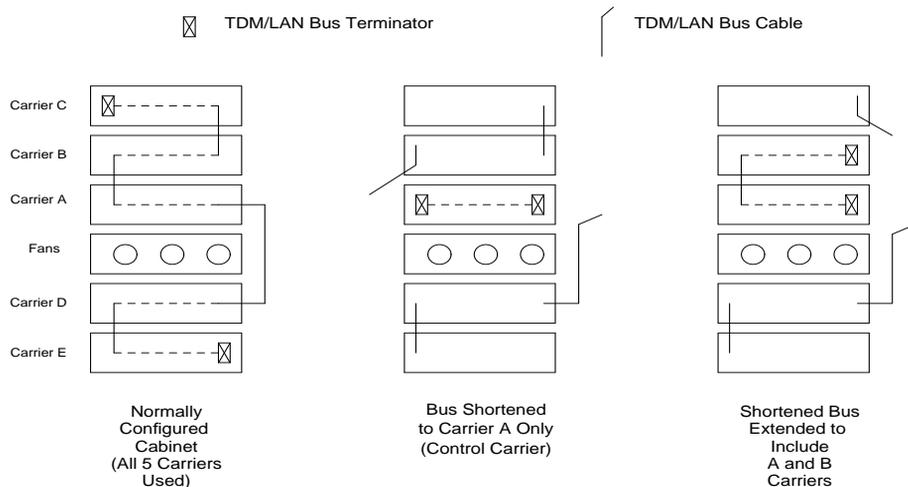
**Figure 5-16. Carrier Rewiring Example—Rear View of Multicarrier Cabinet**
