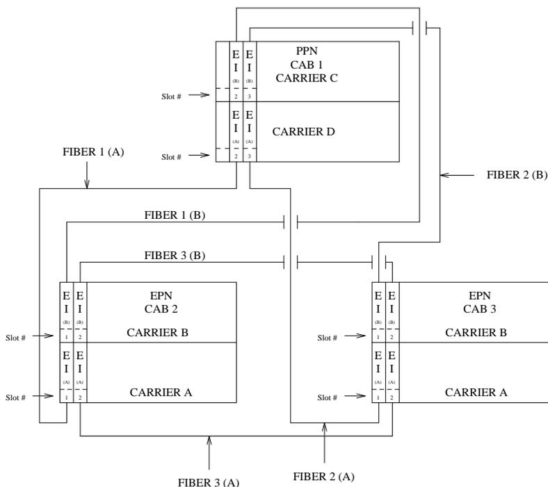
**Figure 9-28. Direct Connect Configuration with Duplicated PNC**
