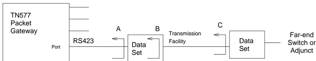
**Figure 9-62. Packet Gateway Port Remote Loop-Around Test**
