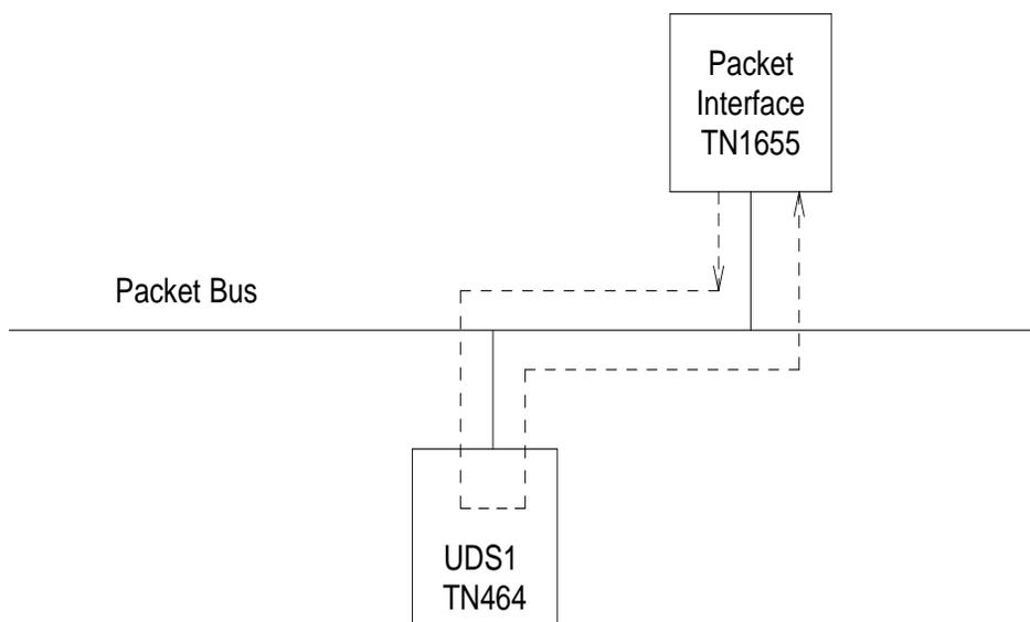
**Figure 9-41. Signaling Port LAN (Packet Bus) Loopback**
