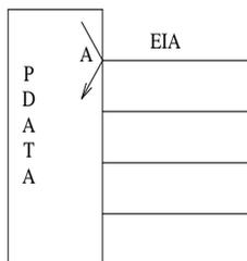
**Figure 9-56. Configuration for Port Local Loop-Around Test**
