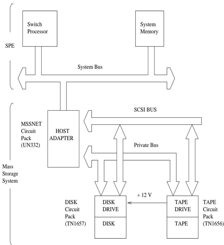
Figure 9-88. Mass Storage System Interactions
