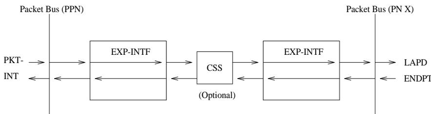
**Figure 9-37. Expansion Interface Packet Interface Test—Packet Endpoint Loop**
