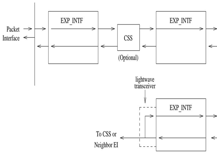
Figure 9-36. Packet BUS Lightwave Transceiver Looparound—EPN only
