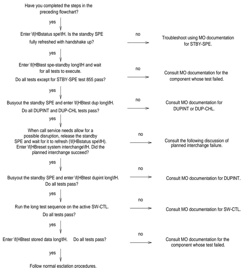
Figure 5-3. Testing the Standby SPE
