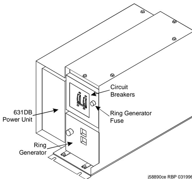
**Figure 9-7. AC Power Distribution Unit (J58890CE-2) — Front**
