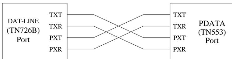
**Figure 9-54. System Port Wiring Scheme**
