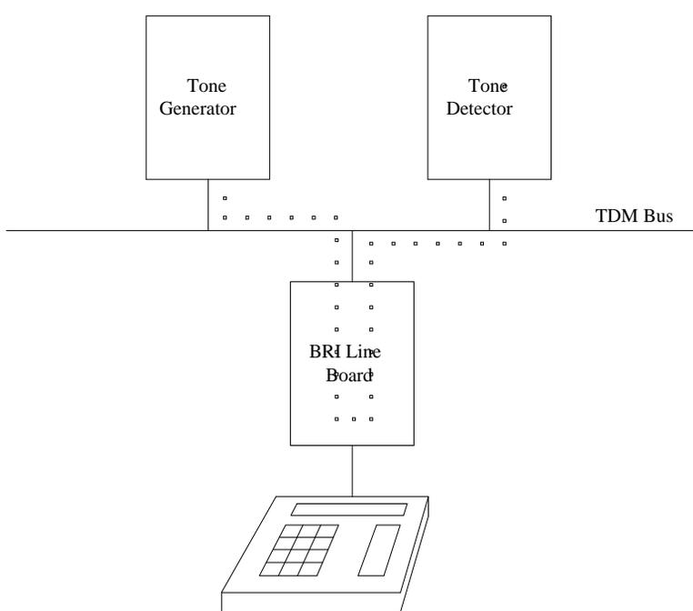
**Figure 9-5. Path of the BRI Port Local TDM Loop Around**
